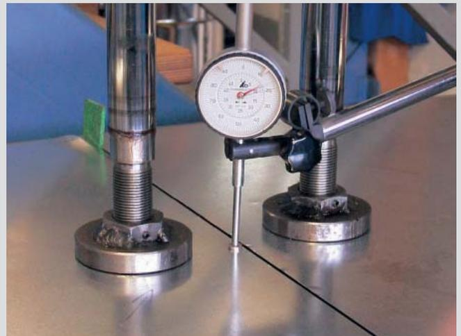
To determine the point load, a static load (such as a table leg) is simulated. On the basis of the permissible point load thus established, the system is generally assigned an appropriate load and deflection class. In accordance with standard practice, the load is applied with a 25 mm x 25 mm indenter.
